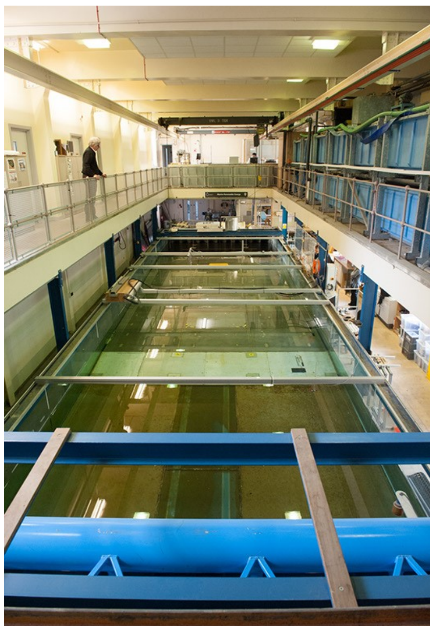
Figure 7. Belfast Wave Flume with an operating depth up to 0.8 m and a 6-paddles Edinburgh Design Ltd Wave Maker with active wave absorption, which can produce regular and random waves up to 0.55 m high
