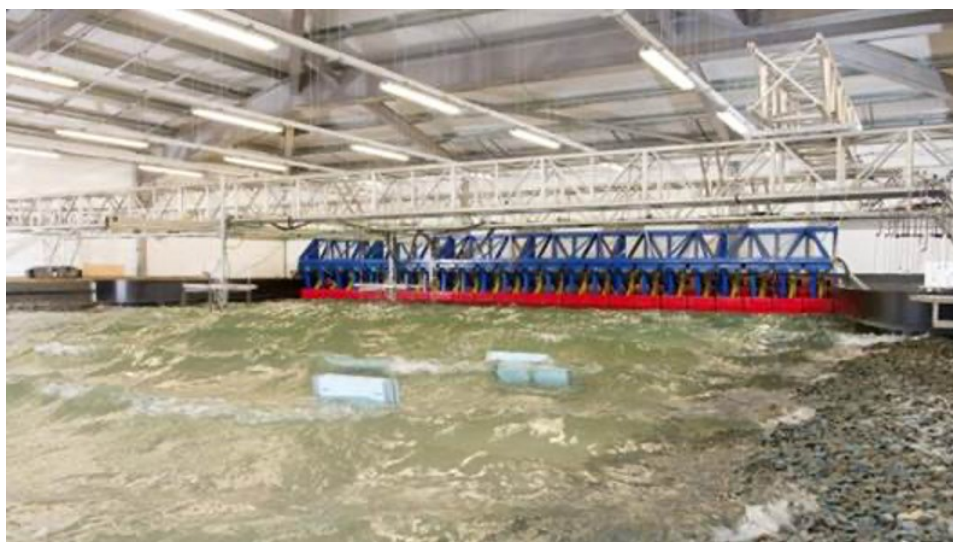
Figure 8. Portaferry Coastal Wave Basin (18 x 16 m) with an operating depth up to 0.65 m and 24-paddles Edinburgh Design Ltd Wave Maker with active wave absorption
