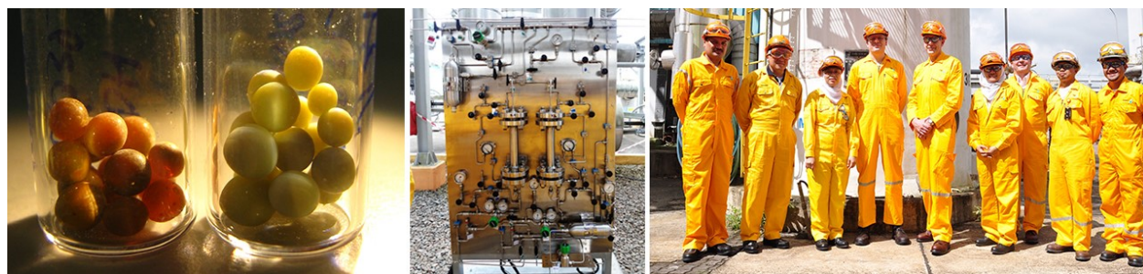
Figure 9. QUB/Petronas Removal of mercury from natural gas streams. Left to right: Mercury removal ionic liquid containing material; pilot plant (QUB/Petronas); Queen's University Ionic Liquids Laboratory/Petronas team in front of the newly developed Hycapture-Hg™ process at Petronas.
