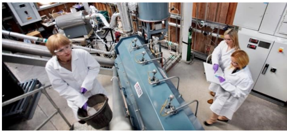
Fig. 6a) Pilot Pyrolysis facility of the UKBRC for generation of experimental biochar/fertiliser.
