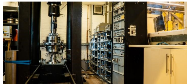
b) The 'true triaxial' GREAT cell (centre left), contained in the loading frame of the 'Big Rig'
