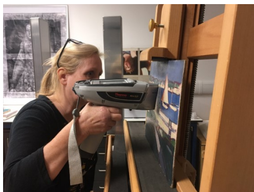
Figure 1. X-Ray Fluorescence identification of pigments on The Hunterian Scottish colourist painting, Royan, 1910 by J. D. Fergusson, in the Study Centre at Kelvin Hall
