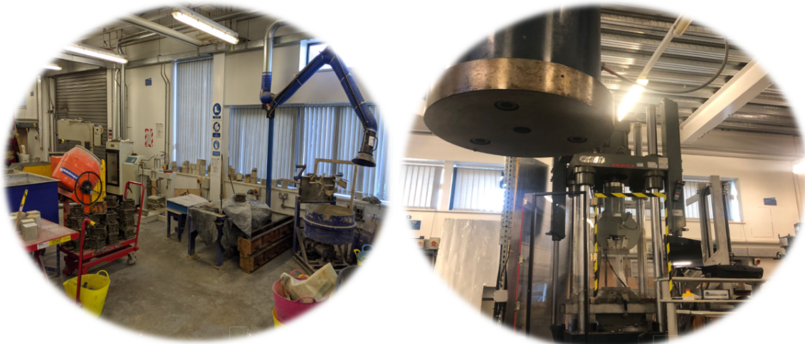
Mixers, Moulds, Vibrating Tables, Curing Tank and 3000kN Compression Machine
