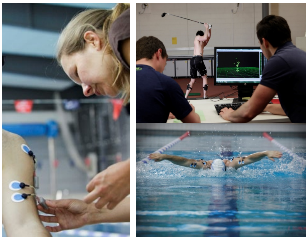
Figure 2: Investment in cutting-edge technology and software, such as the 3-D motion capture system (top right panel) and wireless EMG being demonstrated in our unique “wet lab” facility (bottom and left panels)
