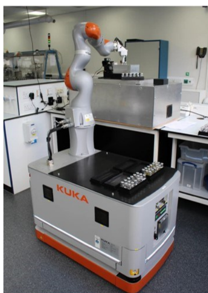
Figure 5 Smart Autonomous Mobile Robot Performing Photocatalyst Discovery Without Human Guidance (Figure adapted from https://doi.org/10.1038/s41586-020-2442-2 )
