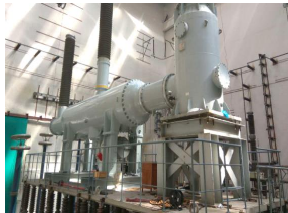
Figure 2: A new design of a single-phase of the 1100kV circuit breaker at Pinggao, enabled by the use of Liverpool's digital design tool. It has dimensions of [text removed for publication] m (length by width by height).
