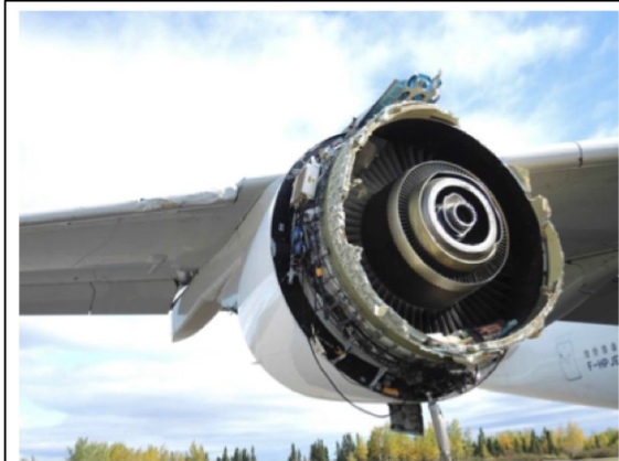
Uncontained engine failure [E1] causing emergency landing of an Airbus 380 flight in Goose Bay, Canada in 2017. Uncontained failure can compromise the aircraft. The flight carried 521 passengers and crew. The failure was demonstrated to be cold dwell fatigue. Our research prevents this kind of catastrophic failure which has been avoided in Rolls-Royce engines.
