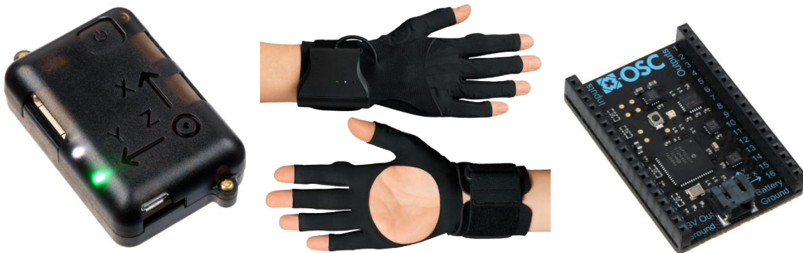
Figure 1 NGIMU (left), MiMU Gloves (centre) photograph Nathan Gallagher, x-OSC (right)
