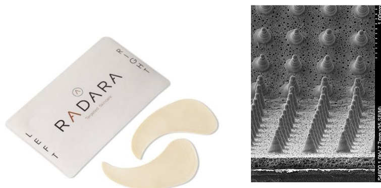
Fig.1. Radara® patches (left) and electron micrograph of microneedles (right)
