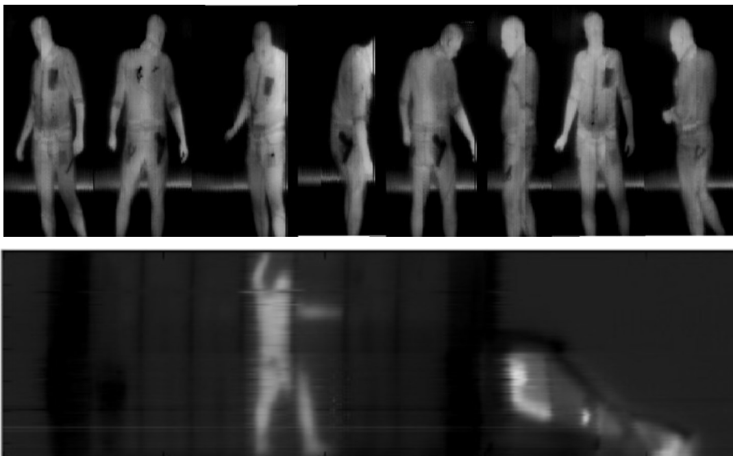
Figure 1. Top: Example output (frame captures) from the Sequestim personnel camera system, showing a variety of hidden threat items. Bottom: Example of an image taken with the truck scanning application. The image was taken of an occupant concealed inside the cargo area of a truck, as it drove past at 30 mph. Note the detection of a gun in the occupant's pocket.
