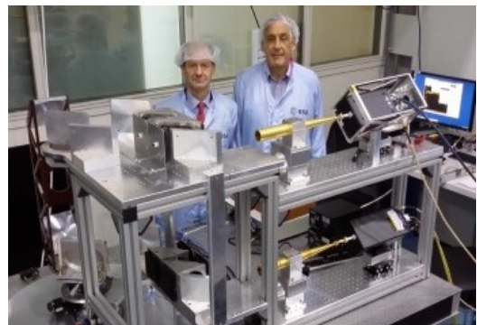
Quasi-optical scatterometer delivered to ESA showing two gold plated ultra-Gaussian horns.
