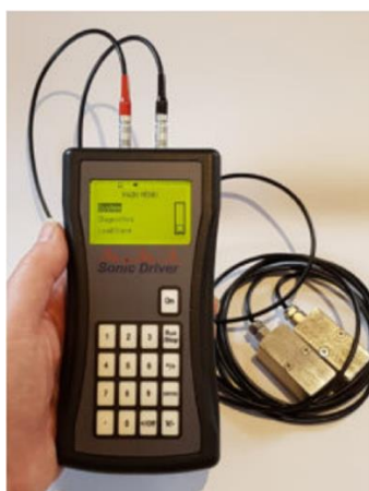
Fig. 4 Sonic Driver’s industry-leading hand-held ultrasonic flow meter, with typical accuracy better than 1.5% - the most compact unit available prior to Sonic Driver’s Android device.
