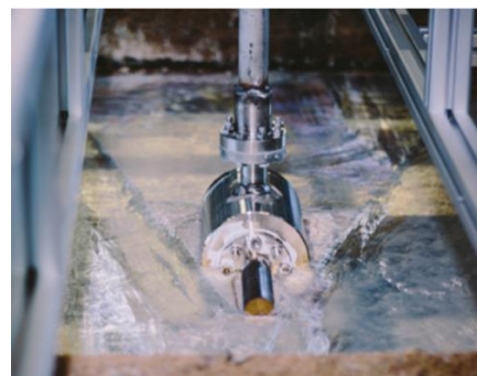
Fig. 3 A high temperature ultrasonic ZIP probe, developed by Sonemat and Zinco, submerging into molten zinc to measure kettle tank wall thickness.
