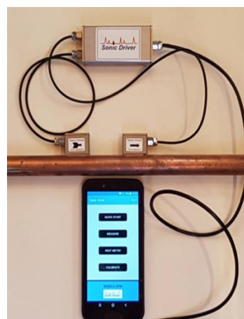
Fig. 5 The world’s first Android clamp-on ultrasonic flow meter, announced in 2020 by Sonic Driver, bringing ultrasonic flow measuring to the mass market without compromising on performance or accuracy.
