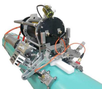
Fig. 2 Sonemat EMAT built into a robotic crawler for pipe testing.
