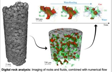
Digital rock analysis: Imaging of rocks and fluids, combined with numerical flow modelling to design improved hydrocarbon recovery and carbon dioxide storage.
