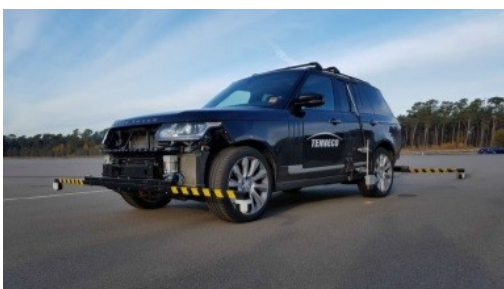
Figure 2 – Demonstrator vehicle by Tenneco with tyre force-vectoring control (left) and example (right) of the enhanced sideslip angle ( \beta_{RA} ) damping performance of the controlled (Active) vehicle with respect to the passive (Baseline) vehicle [R2].
