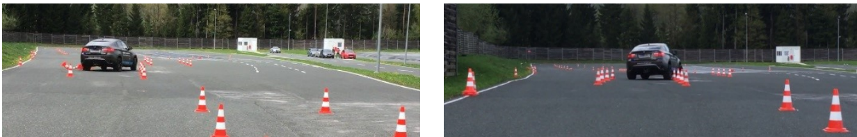
Figure 1 – Obstacle avoidance test performed with the Elaphe's BMW X6 prototype with in-wheel powertrains, without (left) and with (right) the torque-vectoring controller developed by the Centre for Automotive Engineering, from the same initial speed.
