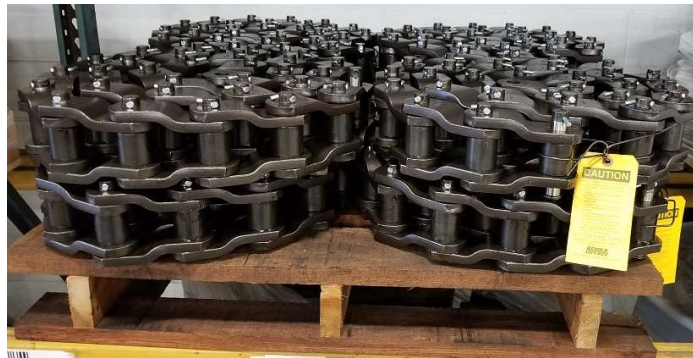
Figure 2. Large industrial drive chain, typically used for heavy construction and mining equipment (4 inch pitch and 4.5 tonne working load)
