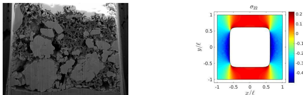
Figure 1: Left, an SEM image of the complex microstructure within an electrode that is distilled into a scalar parameter by Foster's methods (R8). Right, stresses around an electrode particle, predicted in-silico by Foster's model (R2).
