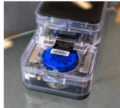
DNAudge point-of-care platform and test cartridge for rapid, lab-free COVID-19 testing.
