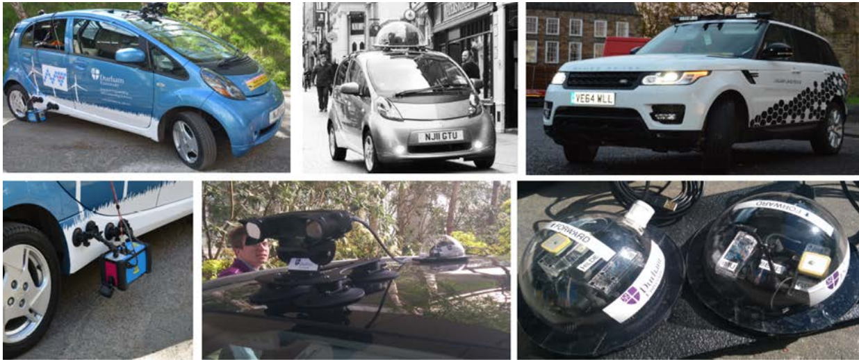
Figure 2: Exemplar on-vehicle sensor rigs used to support data collection and research under [R1-R6] in collaboration with Machines with Vision (left top/bottom), ZF Race Engineering (top middle), Jaguar Land Rover (top right) and Renault (bottom middle/right) – on test at Durham University.
