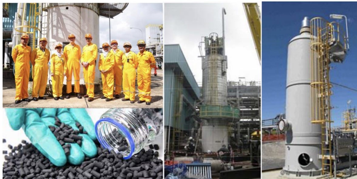
Figure 1: Team at the plant (top left), material coated with Hycapure (bottom left), and two Mercury Removal vessels loaded with 15t SSIL installed at onshore and offshore facilities (middle, right).
