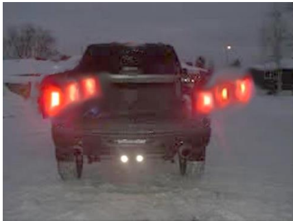
Figure 2. Another temporal light artefact example: tail lights. (Source: https://sudonull.com/post/18780-Brightness-pulsations-facts-mechanisms-and-norms )
