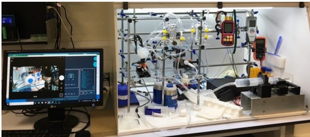
Vaping and smoking simulator at the University of St Andrews
