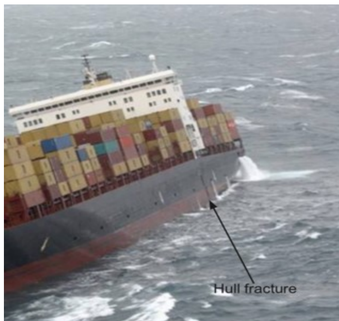
Figure 1: Damage to the Hull of MSC Napoli.
