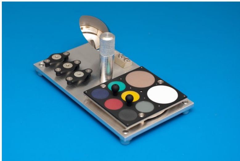
Figure 2: ExoMars PanCam ‘Small Items’ Engineering Model (image courtesy of M. de la Nougerede, UCL/MSSL)
