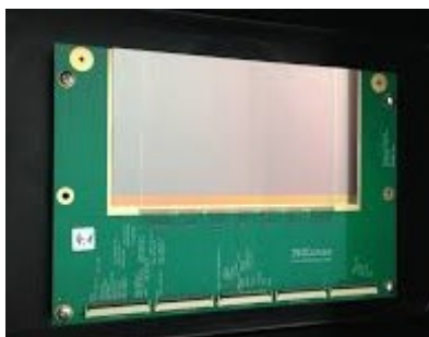
PRaVDA CMOS Sensor - 10 cm x 5 cm Radiation-hard and 1,000 frames per sec, for direct detection of protons
