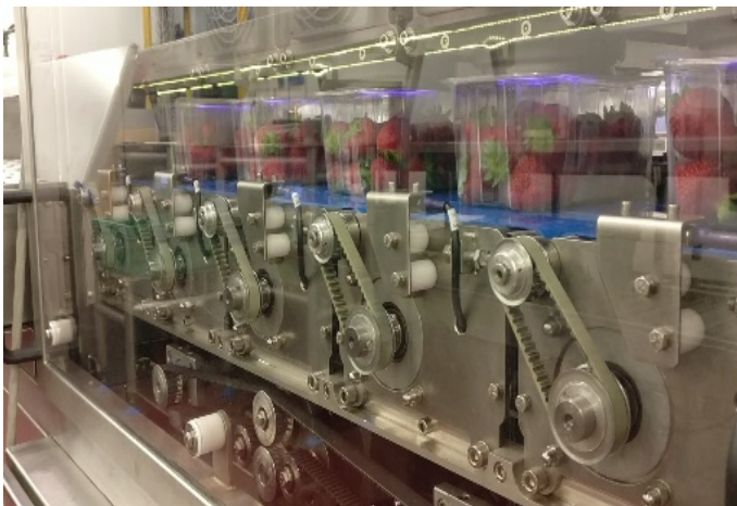
Anacail 10-head 120 packs/minute machine in factory showing plasma glow in packaged fruit
