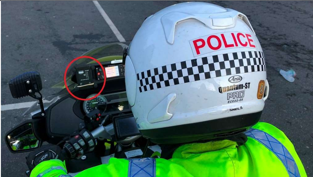
Chronos CTL3510 jamming detector fitted to a police motorcycle.
